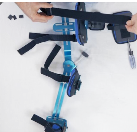
Estimate the length of the thigh strap by adjusting the tri-glide buckles.
